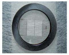
Two wire prototypes 100  $\mu$ m wide, 3  $\mu$ m thick and 11 mm high have been already realized. One of them is shown in the figure.
