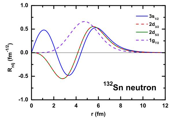
\* Single-particle wave functions of the  $3s_{1/2}$ ,  $2d_{3/2}$ ,  $2d_{5/2}$ , and  $1g_{7/2}$  states.
