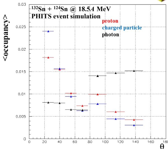
**Si-CsI detector unit coverage of polar angle tuned to be  $\langle \text{occupancy} \rangle < 0.1$**
