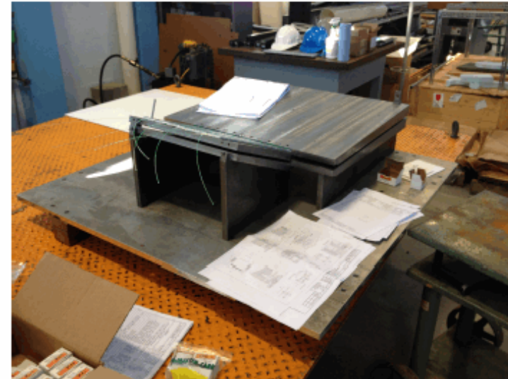
Figure 3.32 HCal prototype under construction. The first layers of absorber are being stacked on the lift table for the beam test.
