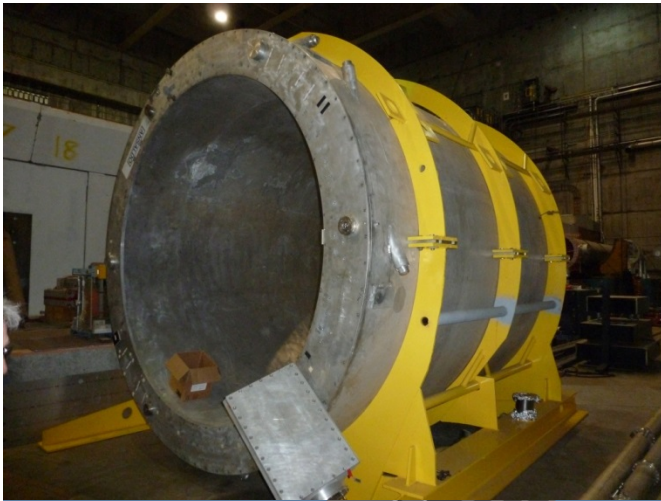
BaBar Magnet from SLAC : 1.5 T solenoid Inner / outer radius / z-length : 140 / 173 / 385 cm
