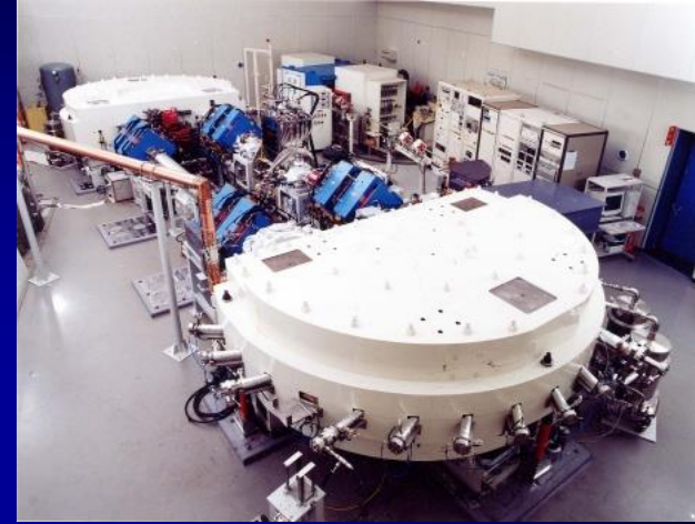
Synchrotron & Storage Ring AURORA (700MeV)
