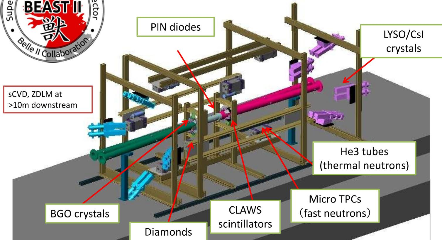
Various measurements (fast charged particle, high-energy photons, thermal/MeV neutron, dosimetry, etc..) to **validate beam loss simulation**
