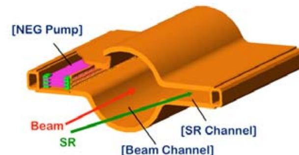
New TiN-coated beam pipe with antechambers
