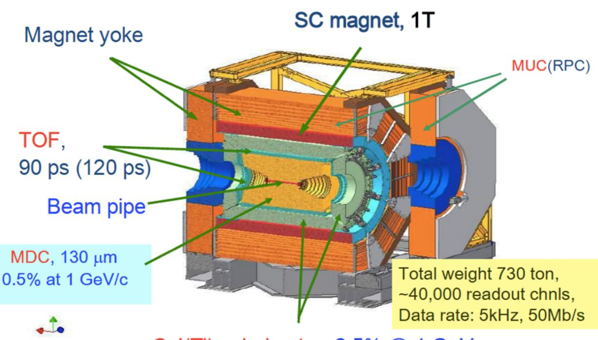
CsI(TI) calorimeter, 2.5% @ 1 GeV
