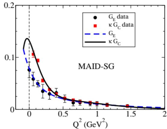
MAID-SG parametrization:  $G_D = (1 + Q^2/0.71)^{-2}$ ,  $C_0 = \frac{1}{e} \left( \frac{M^3 K}{M_R} \right)^{1/2}$
