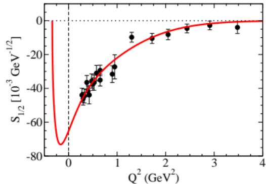
Jlab-SG parametrization (fit to Jlab data):  $D = K / \sqrt{Q_+^2}$  ST  $\rightarrow b_0, c_0$
