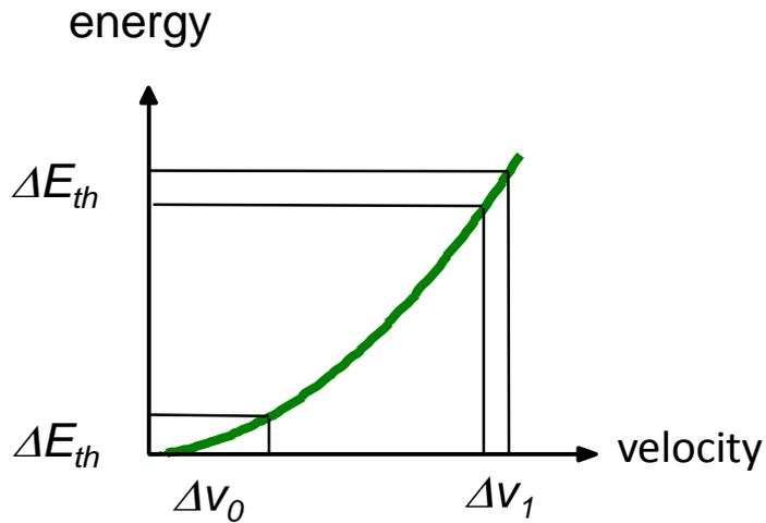
$$\frac{\Delta v_1}{\Delta v_0} = \sqrt{\frac{kT}{eU}}$$
