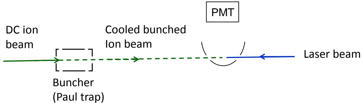
$$\text{Noise Reduction} = \frac{\text{Bunched Noise}}{\text{DC Noise}} = \frac{\text{Pulse duration}}{\text{Time between pulses}}$$
