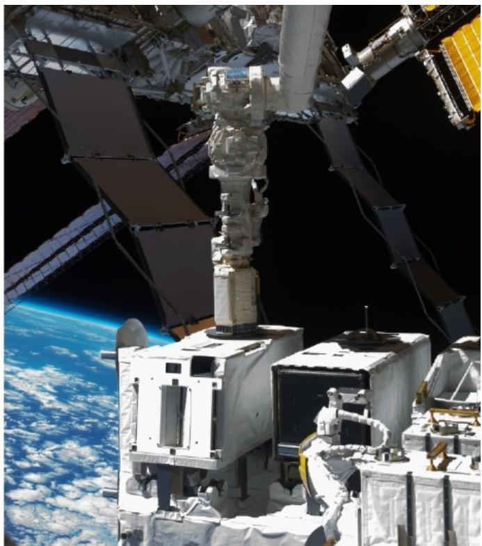
2009/7/23 Astronaut Wakata-san at ISS moved robot-arm to mount MAXI at JEM-EF port.
