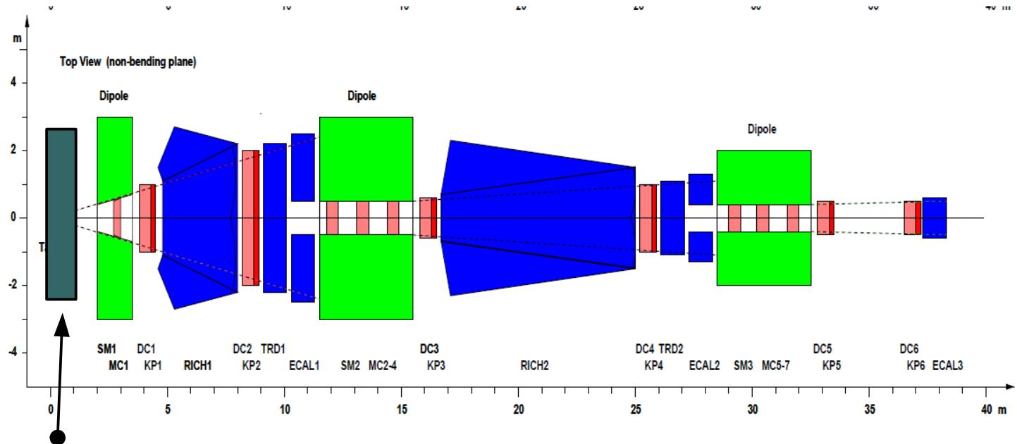
Figure 3.3.2: Schematic side view and top view of the envisaged TESLA-N apparatus. For text.
