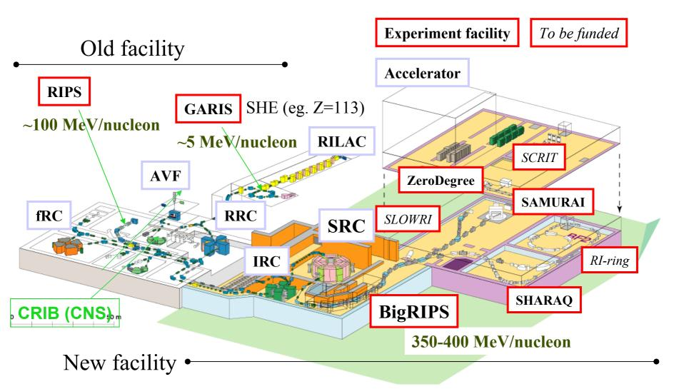
Intense (80 kW max.) H.I. beams (up to U) of 345AMeV at SRC Fast RI beams by projectile fragmentation and U-fission at BigRIPS Operation since 2007
