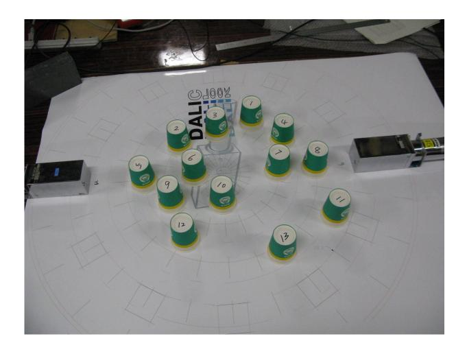
Two detectors lie on a line and rotate clockwise along the circle
