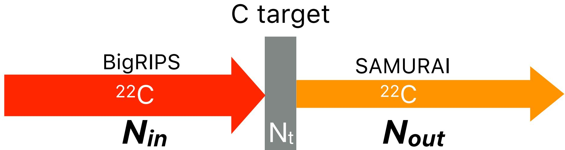
$$\sigma_I = -\frac{1}{N_t} \log \left( \frac{\Gamma}{\Gamma_0} \right) \quad \Gamma = \frac{N_{out}}{N_{in}}$$
