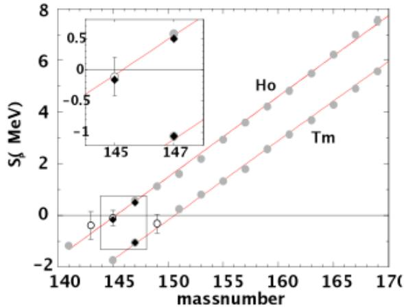
SHIPTRAP: First direct mass measurement beyond the proton dripline.
