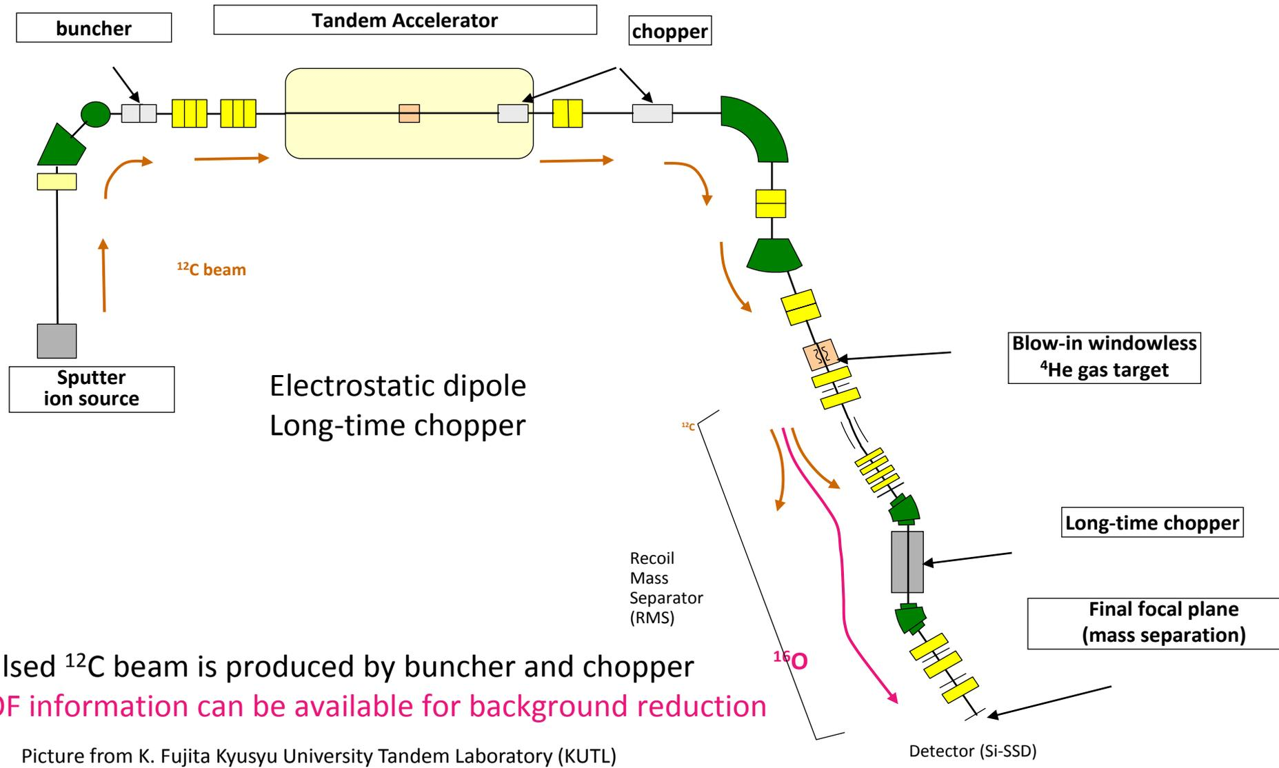
Pulsed  $^{12}\text{C}$  beam is produced by buncher and chopper
