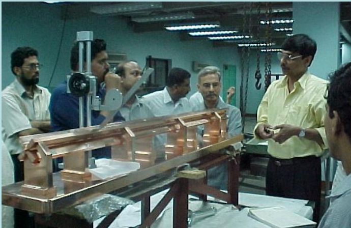
CMERI Durgapur – RFQ vanes, posts
