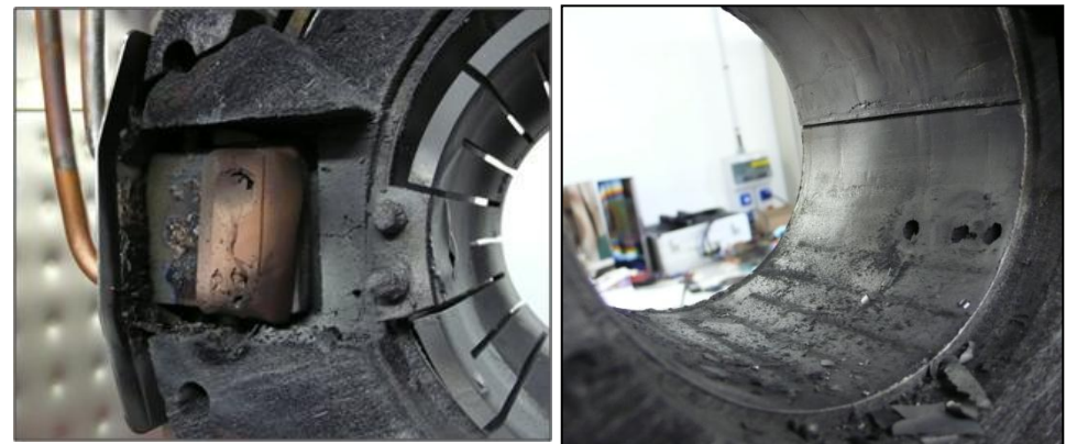
Some contact has caused local over-heating
