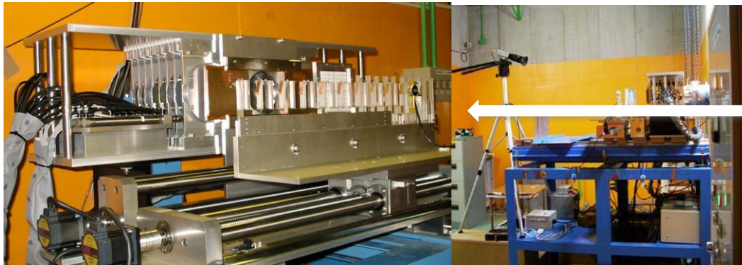
Ver.2 model of Apr. 2003 (12 samples/h) with the range shifter (LET adjuster)
