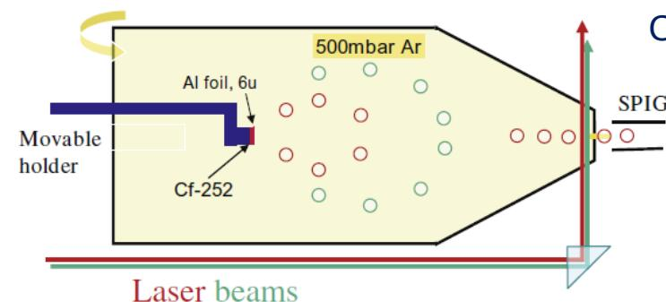
Characterization of the gas cell with a 0.78 mCi  $^{252}\text{Cf}$  source
