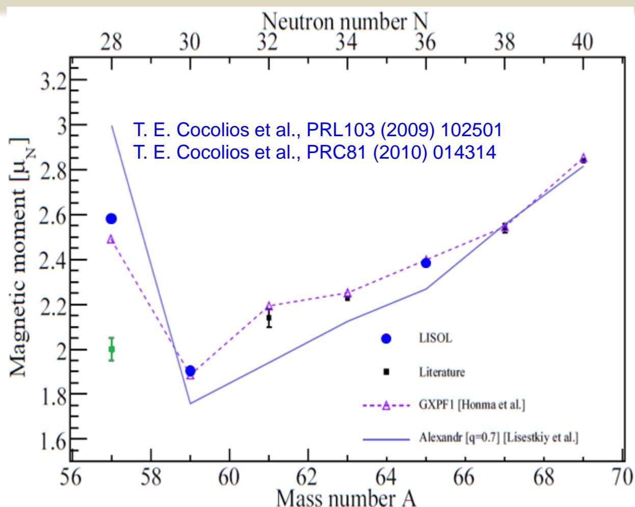
Magnetic moment of  $^{57}\text{Cu}$  isotopes using the  $\beta$ -NMR technique
