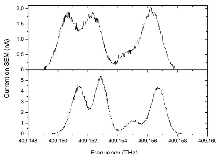
First step scanning of  $^{63}\text{Cu}$
