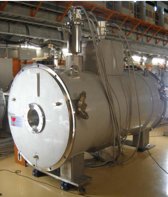
Fig. 6. A schematic diagram of the prototype quadrupole triplet with small cryocoolers.
