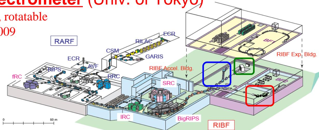
RIBF RI beam generator featuring superconducting ring cyclotron (SRC) and projectile fragment separator (BigRIPS) will be commissioned late in 2006.
