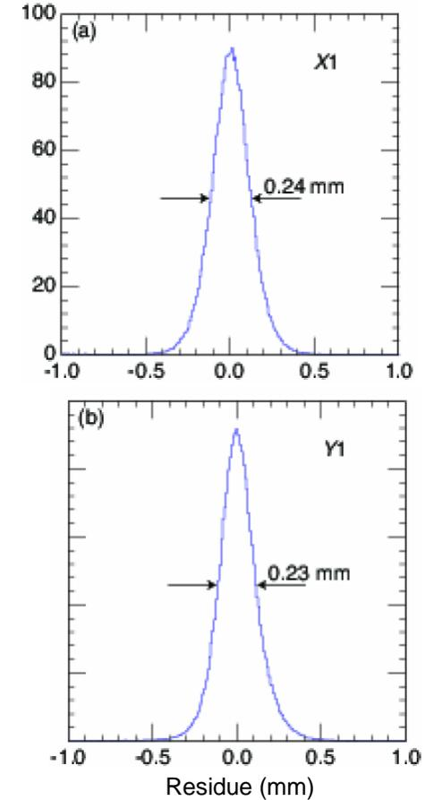
Evaluation of Position resolution for  $^{12}\text{N}$  particles.
