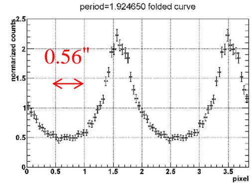
MIXIM succeeded in **sub arcsecond X-ray Imaging** with a grating and a CMOS pixel detector separated by 46cm.
