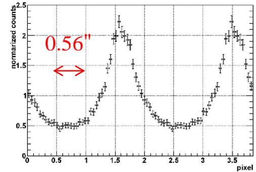
MIXIM succeeded in **sub arcsecond X-ray Imaging** with a grating and a CMOS pixel detector separated by 46cm.
