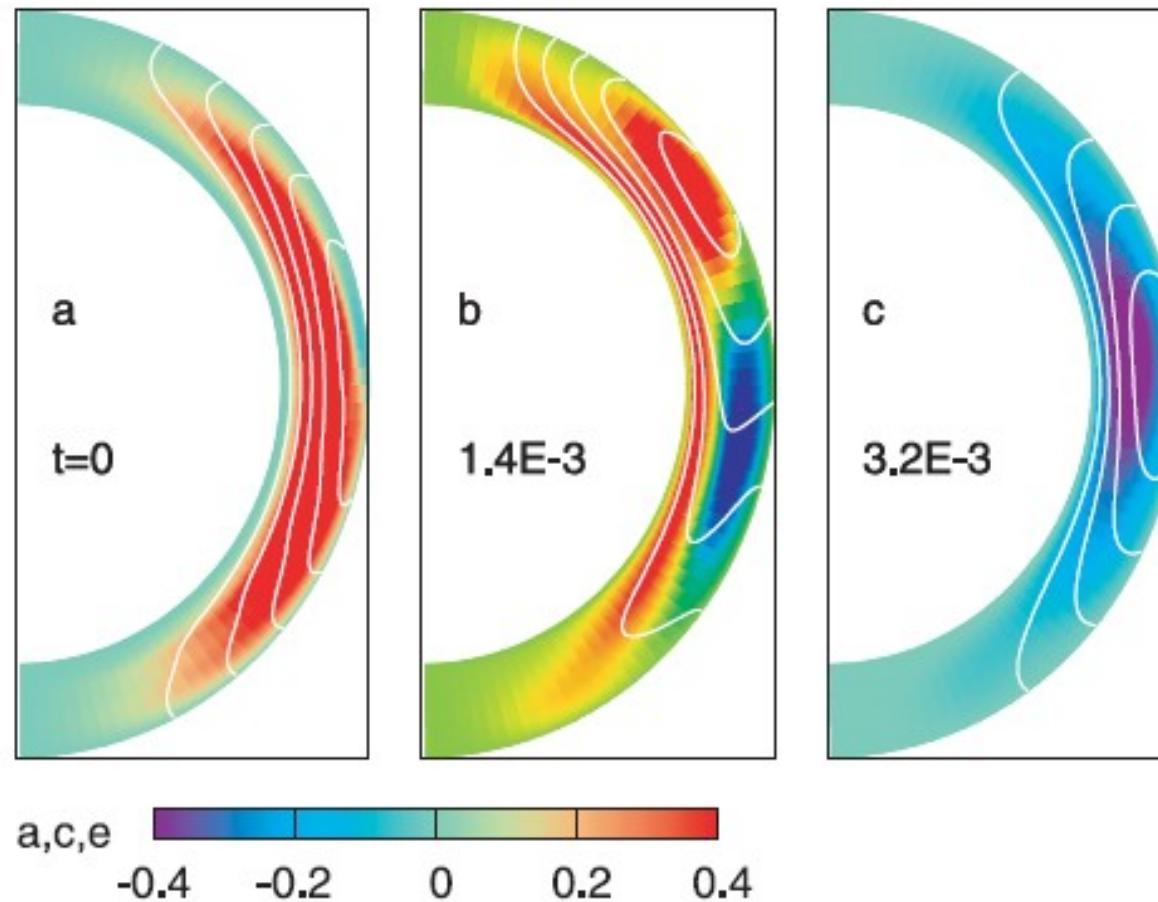
Toroidal field is transformed into the higher order poloidal fields.
