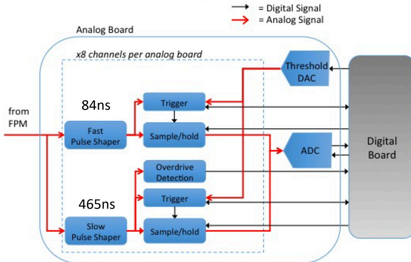
Figure 5. Analog board functional diagram.
