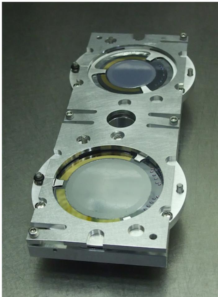
Two filters installed in mounting fixture.
