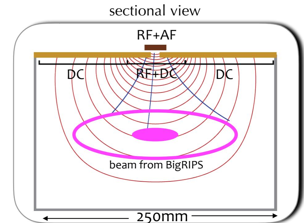
Two stage RFcarpet: “Gutter Structure”
