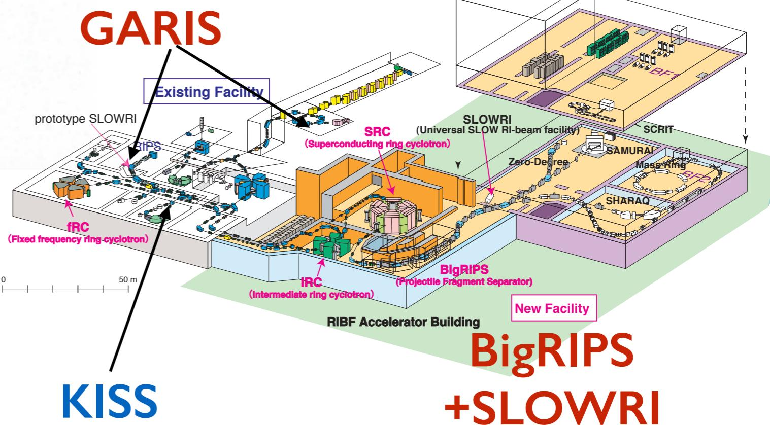
we plan to measure all available nuclides at RIBF, using multiple MRTOF mass spectrographs
