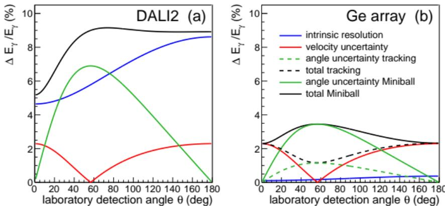
→ MB at forward angles, tracking detectors at 60°
