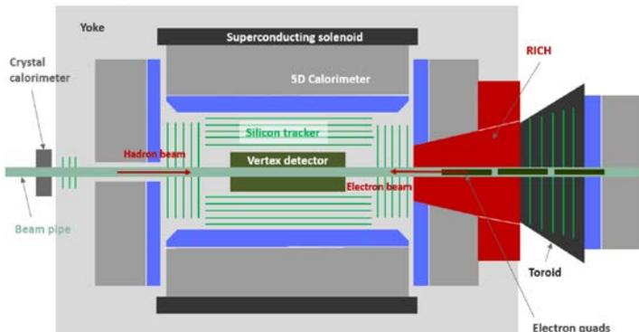
JLEIC Detector Concept with CLEO Solenoid
