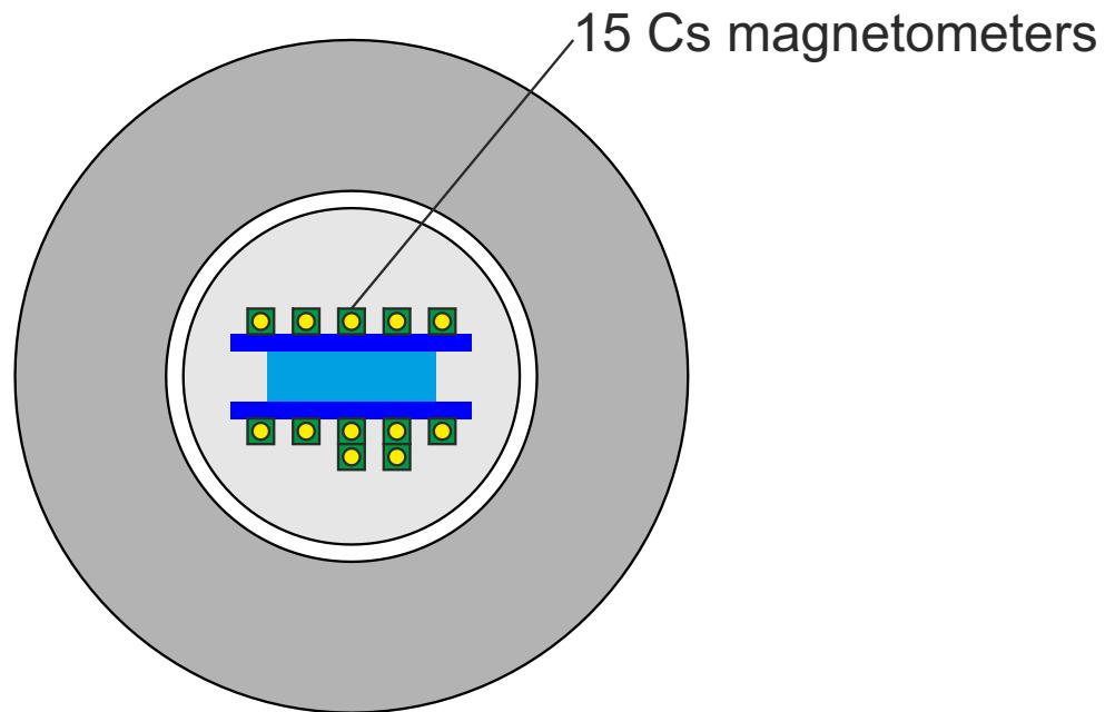
Optically pumped Cs magnetometers enabling a high-sensitivity search for the neutron electric dipole moment, C. Abel et al. PRA 101, 053419 (2020)
