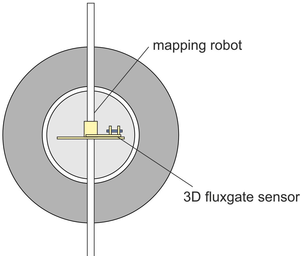
Mapping of the magnetic field to correct systematic effects in a neutron electric dipole moment experiment.
