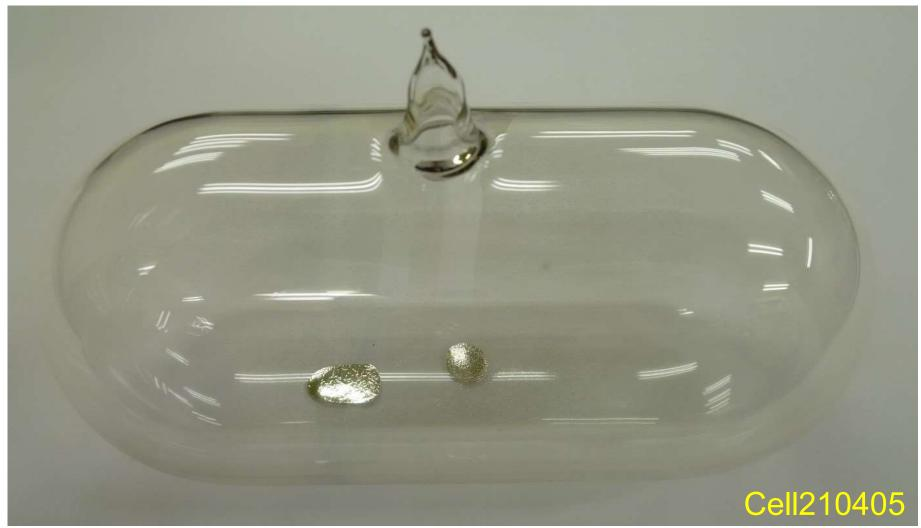
Pyrex glass Diameter : 72 mm Length : 156 mm Wall thickness
