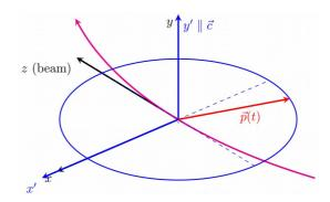
Spin vector that is invariant under one turn spin transfer matrix is called the invariant spin axis
