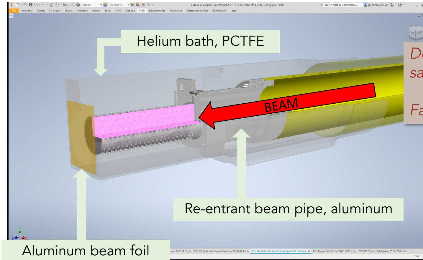
Design of beam-ready bath and sample containers is complete.
