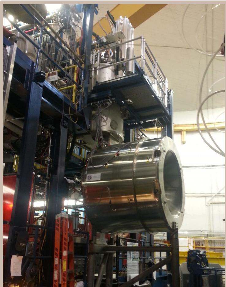
The CLAS12 solenoid will provide the 5 T field for polarizing the target.
