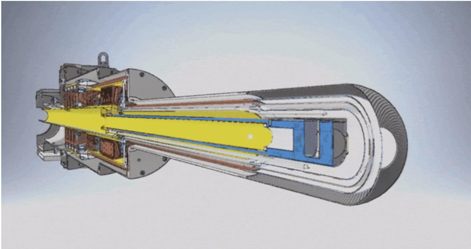
The target bath is retracted to an upstream load-lock position, where an old target sample is removed and replaced with a fresh sample.
