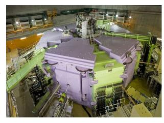
(~10kW) are injected to Fragment Separator called BigRIPS to generate an RI beam for all elements up to uranium with the world-highest intensity. These beams are provided to several experimental systems such as SHARAQ, SAMURAI, ZeroDegree to study nuclear physics and reveal the evolution of the universe. In the tour, we show the SRC and BigRIPS.
