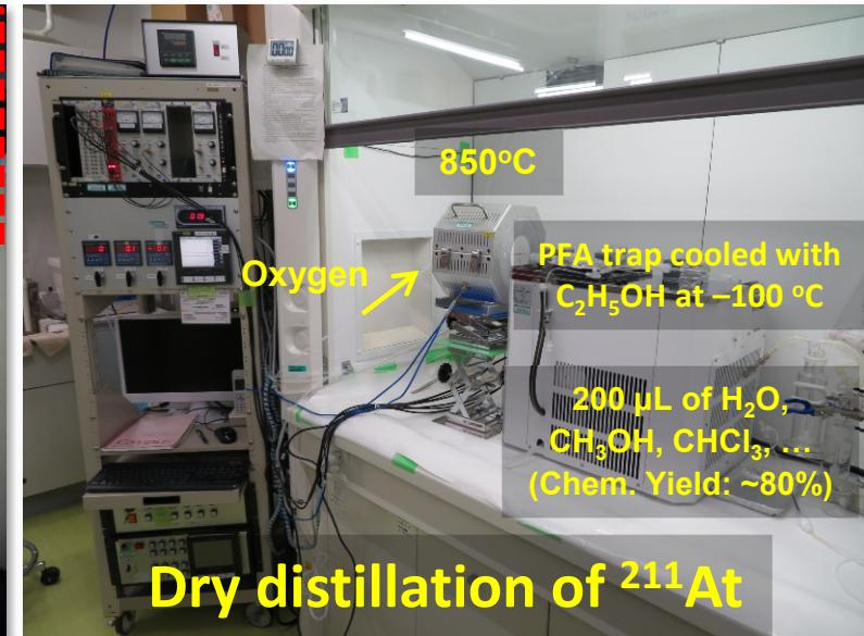
$25 \text{ p}\mu\text{A} \times 1 \text{ h} \rightarrow 1.2 \text{ GBq of } ^{211}\text{At (EOB)}$
