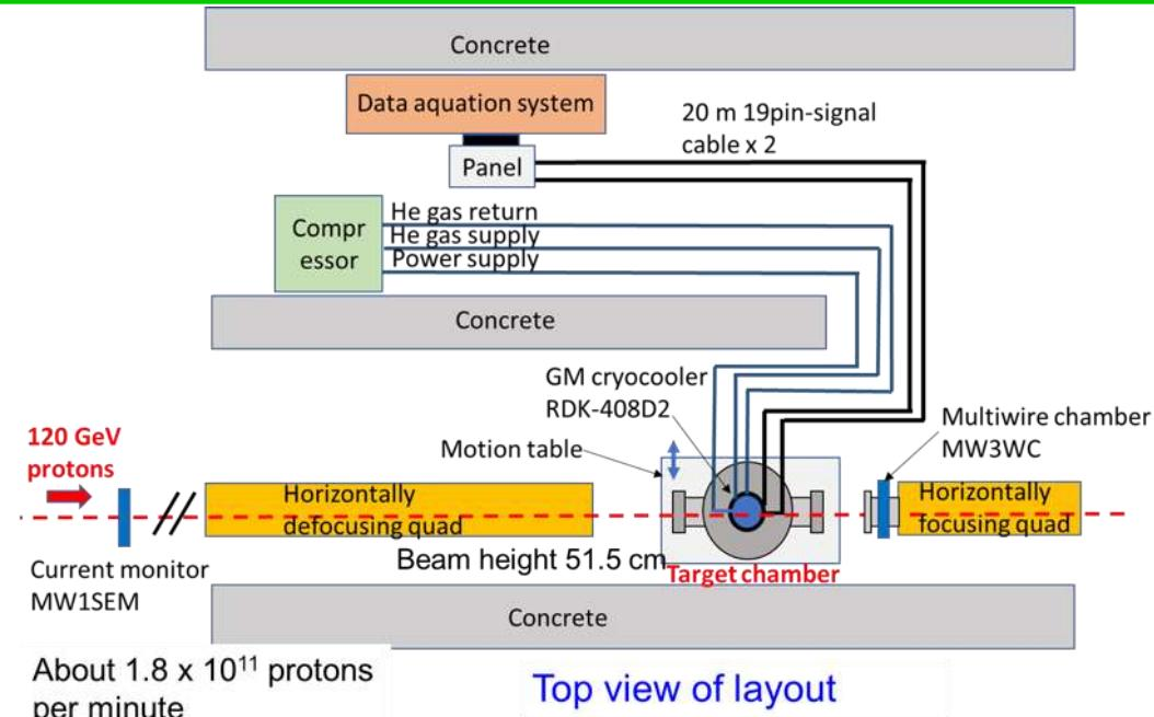
Horizontal beam position and width were scanned by using motion table.
