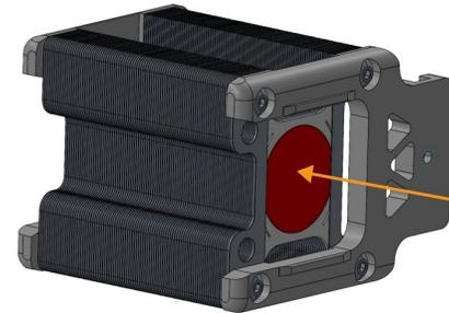
Stack of Mo-100 discs separated by fixed gap
