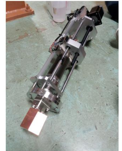
Water-cooled electric slit 1 kW max. for each side
