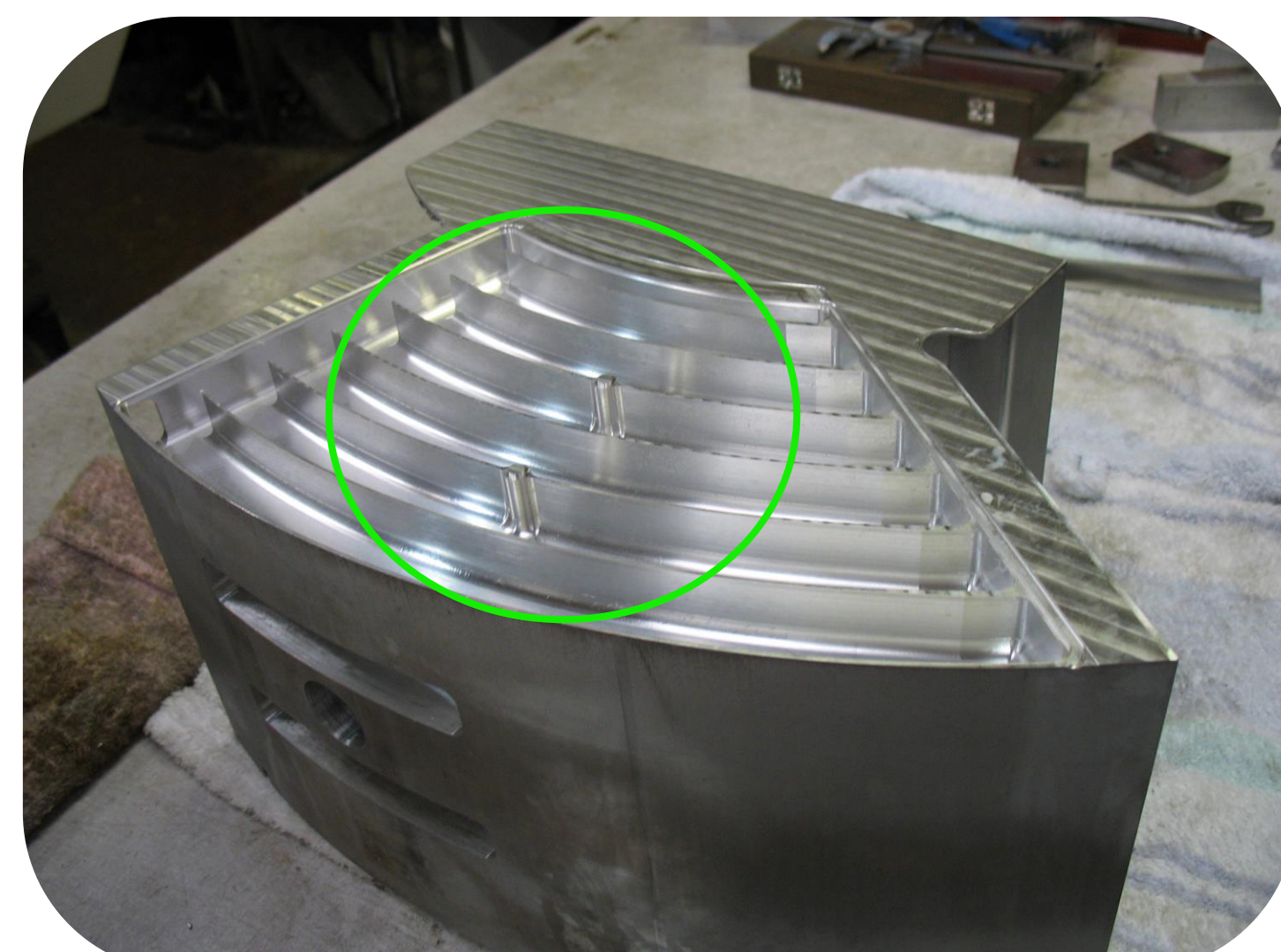
(b) Second iteration with the additional welded "pips" for structural rigidity.
