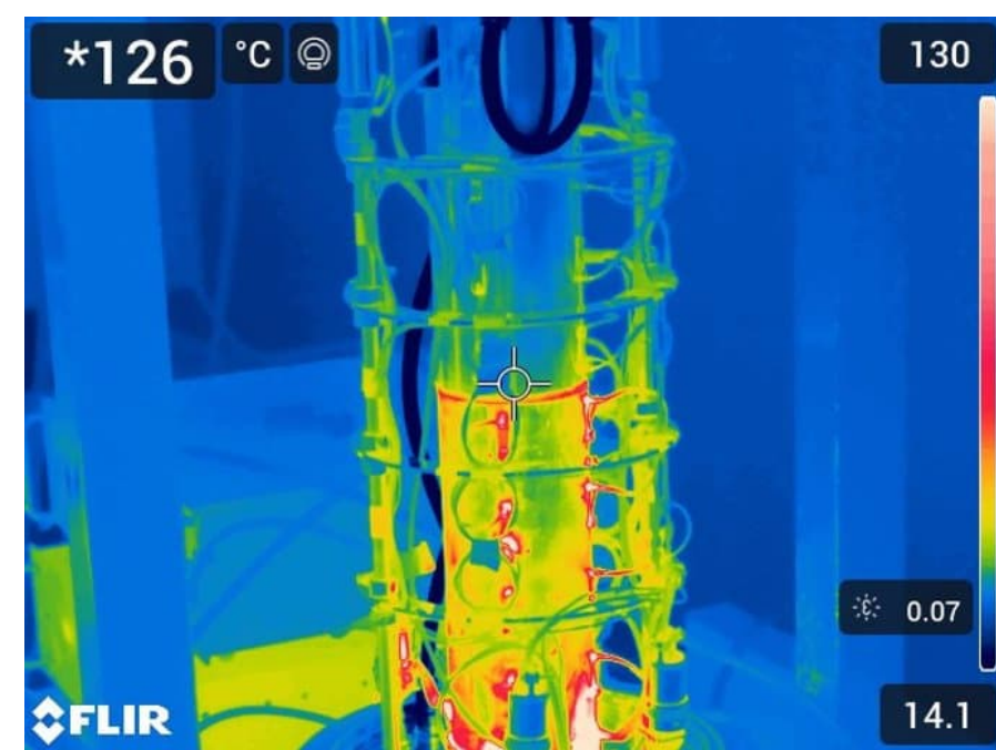
Figure 5: Tantalum and stainless-Steel sample for thermal conductance assessment captured with a thermal camera
