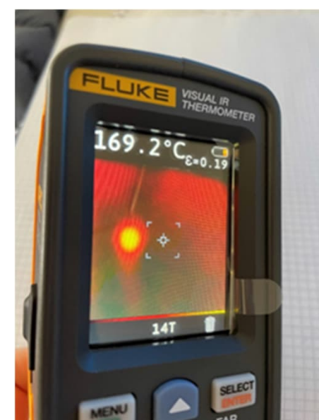
Figure 7: Taking measures with an infrared thermometer, changing the emissivity until having the same temperature
