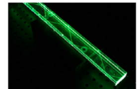
A "mini-DIRC" inside a Roman pot at the downstream focus can identify ions to \sim 1\% in Z^2
