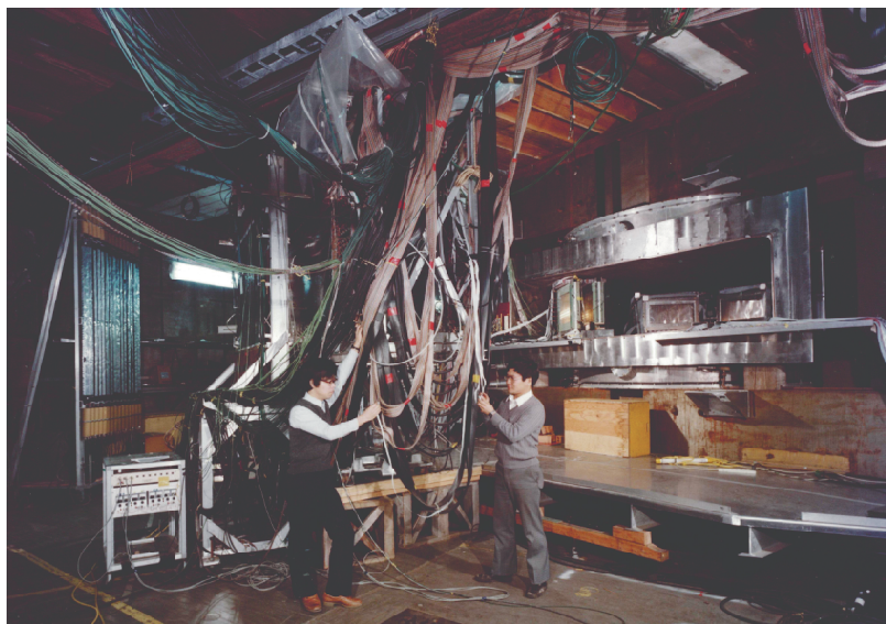
O. Hashimoto / Kobayashi 1983 HISS pion experiment w 2mx1m drift chamber
