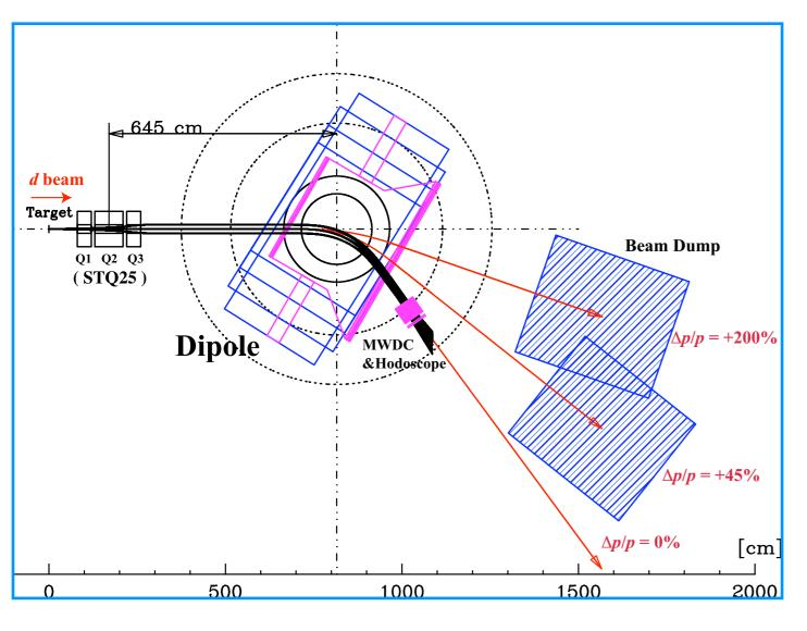
In experiments with polarized deuteron beams high momentum resolution  $p/\Delta p \sim 1600$  for 1.5 GeV/c proton
