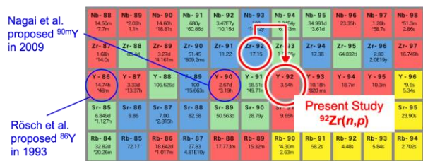
Fig. 2 Production routes of radioactive yttrium isotopes. The ^{92}\text{Y} proposed in the present study can only be produced via the fast neutron-induced method.
