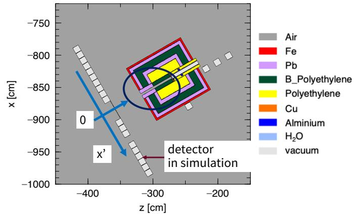
Figure 8: Target station with a BPE + Pb collimator.
