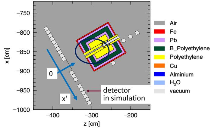
Figure 6: Target station with a PE collimator.
