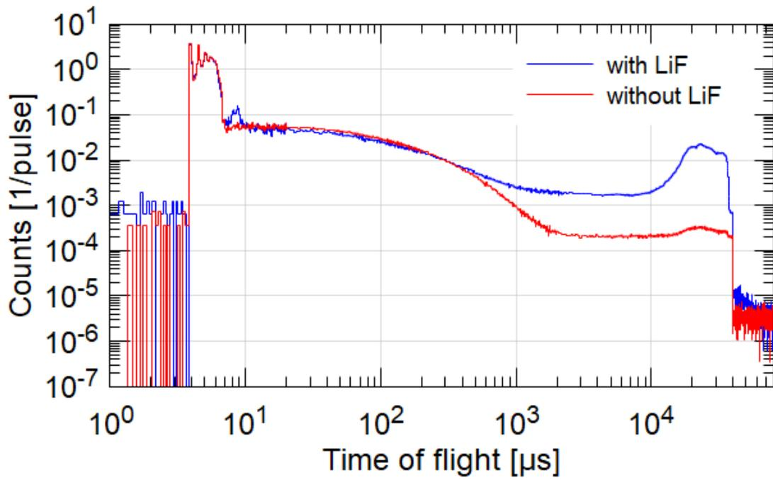
Figure 3: TOF spectra with and without LiF.
