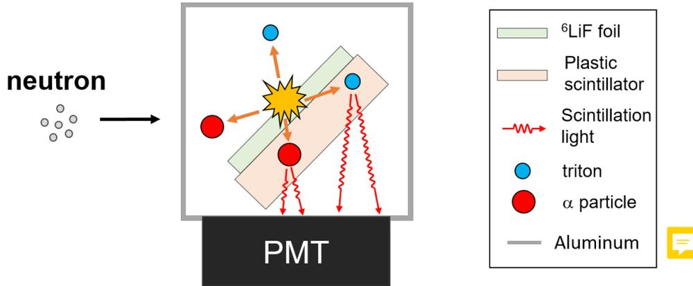
Figure 1: Detector geometric design.
