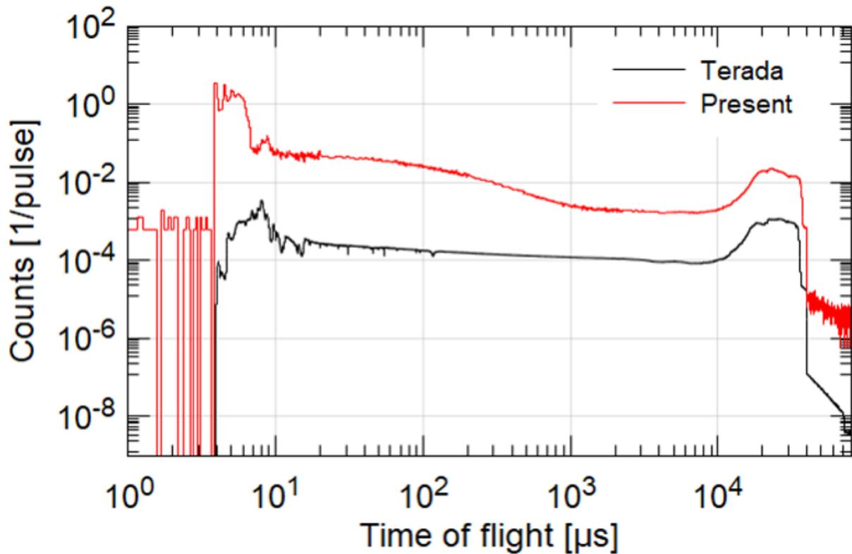
**Figure 5:** Comparison of TOF spectra of the present work with the previous measurement by Terada [4].
