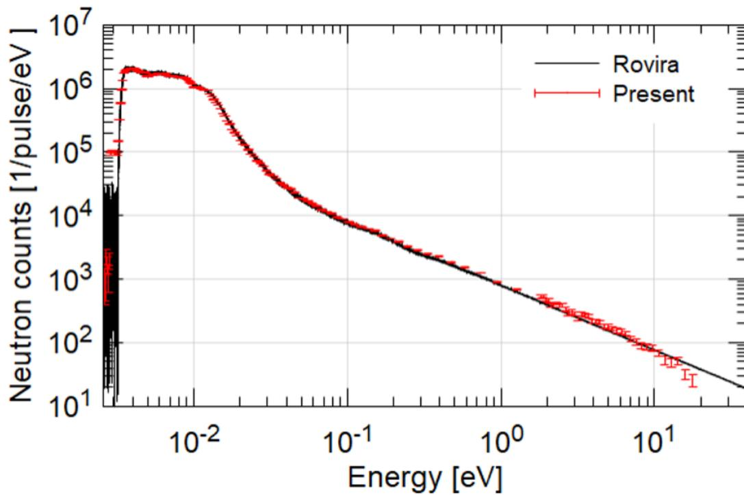
Figure 4: Comparison of neutron spectra of the present work with the previous measurement by Rovira [3].
