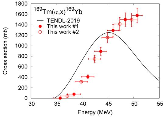
Fig. 4. Excitation function of the  $^{169}\text{Tm}(\alpha,x)^{169}\text{Yb}$  reaction with the TENDL-2019 values [6].
