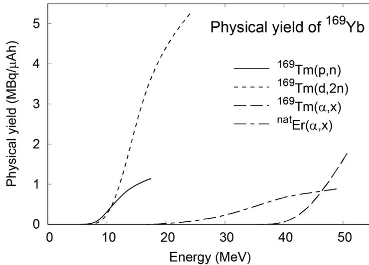
Fig. 6. Physical yields derived from the measured cross sections.
