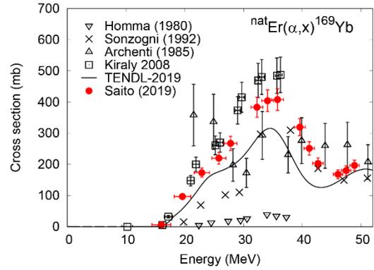
Fig. 5. Excitation function of the  $^{\text{nat}}\text{Er}(\alpha,x)^{169}\text{Yb}$  reaction with the previous data [15–18] and the TENDL-2019 values [6].
