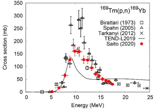
Fig. 2. Excitation function of the  $^{169}\text{Tm}(p,n)^{169}\text{Yb}$  reaction with the previous data [13,14] and the TENDL-2019 values [6].
