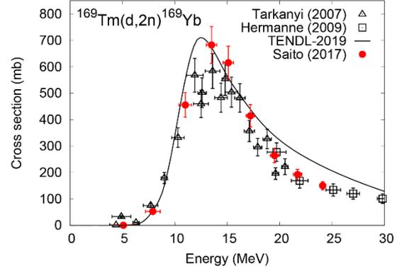
Fig. 3. Excitation function of the  $^{169}\text{Tm}(d,2n)^{169}\text{Yb}$  reaction with the previous data [13,14] and the TENDL-2019 values [6].
