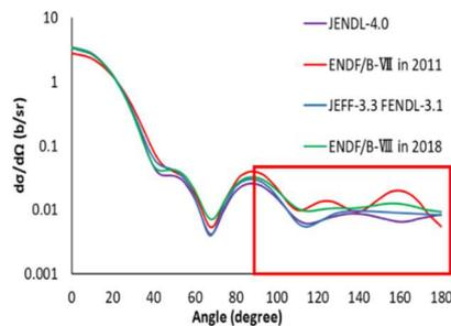
Figure 1 Angular distribution of neutron elastic scattering reaction cross section of  $^{56}\text{Fe}$  at 14 MeV. [4-8]
