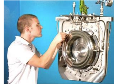
Beam window in neutrino facility (Ti alloy)
